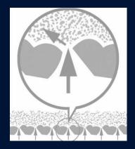
Horizontal air flow enables conveying of the product and supports the discharge at the same time. The direction of the airflow over the distribution plate can be determined by arranging the **CONIDUR®** Pierced Sheet in different ways.
